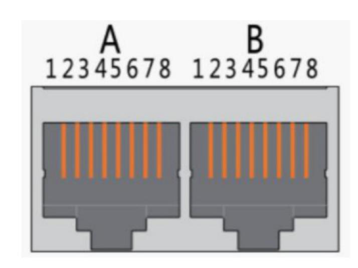
With dual RS485 interfaces, the default baud rate is 9600bps. If you need to communicate the batteries in parallel with the monitoring device or inverter, you need to connect each battery with RS485-2 ports, so the host battery can read the information of each battery.
