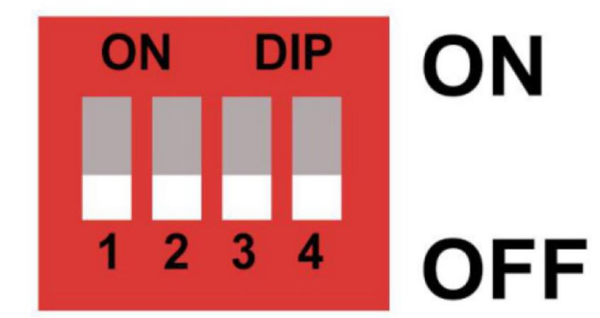
When the battery packs are connected in parallel, the dial code switch of each battery can be used to distinguish different Pack addresses. The hardware address can be set through the dial code switch on the board. The definition of the dial code switch refer to the following table.
